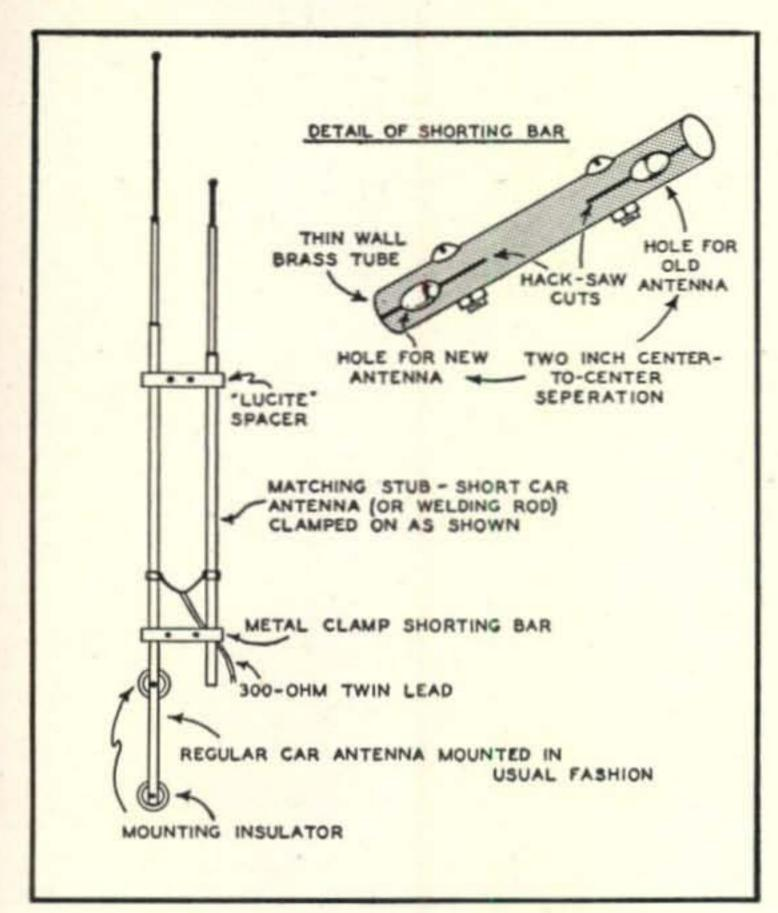
Construction detail of the dual purpose mobile antenna. An extra long whip antenna is used to replace the common shorter variety. The BC connections remain the same, while the mobile rig works into a J-type antenna through 300-ohm feedline.
